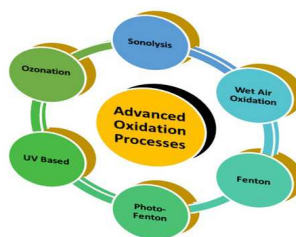
Figure 2. (a) Advanced oxidation processes classification (b) The sorption hysteresis loop
